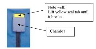
To remove seal lift seal tab until it breaks, remove tab and lift lid of chamber to reveal spent seal legs.
